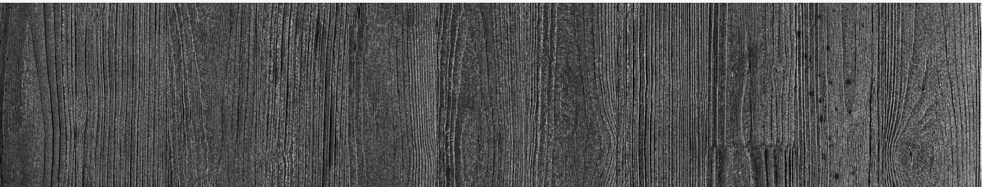
SH162-05 Holz Brettschalung gestoßen SH162-05 Wooden Board Formwork butted
