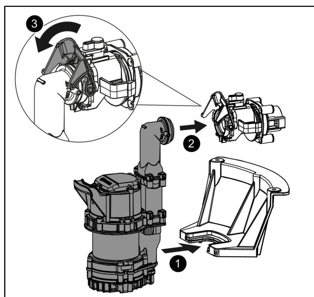
**Installing the level detector (Tronic variants only)**
