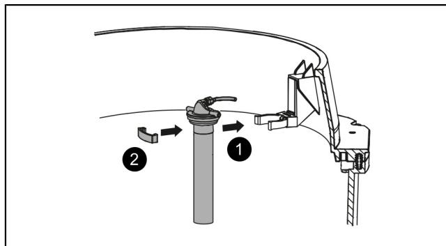
**Fitting the alarm probe (only Tronic variants)**
