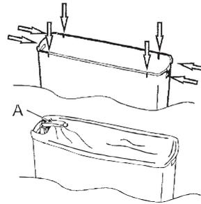
ENSURE BAG IS UNDER PEDAL LEVER (A) TO AVOID OBSTRUCTION. REPLACE COVER.
