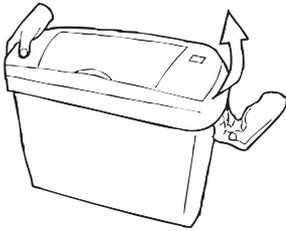
REMOVE TOP COVER BY PULLING ONE SIDE OF COVER UPWARDS.
