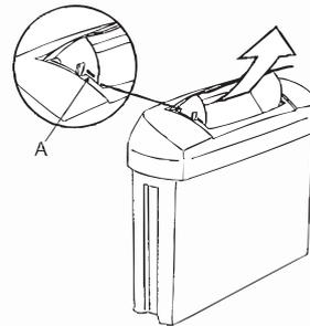
**REMOVING THE FLAP FOR CLEANING**
