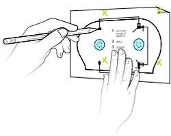
MARK THE POSITION TO DRILL WALL MOUNTING HOLES.
