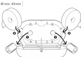
DEPENDING ON THE CORE DIAMETER, REMOVE (Ø MIN. 43 MM) OR ATTACH (Ø 54–70 MM) THE ADAPTER.
