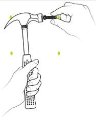
TAP ANCHORS INTO EACH DRILLED HOLE.
