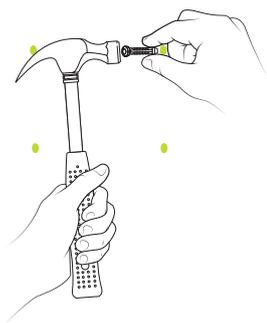
TAP ANCHORS INTO EACH DRILLED HOLE.
