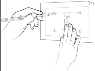
MARK THE POSITION TO DRILL WALL MOUNTING HOLES.
