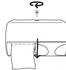
**CLOSE THE DISPENSER AND ENSURE THAT THE LOCKING MECHANISM ENGAGES.**
