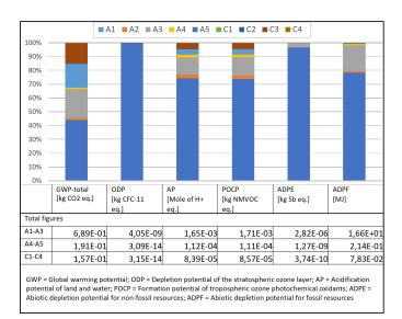
The dominance analysis of the impact assessment indicators shows a large contribution from the manufacturing phase (A1-A3). A large proportion of the environmental impact originates from the raw materials used (A1), with the synthetic polymer dispersions making the highest contributions (with regard to the impact indicator Climate Change -total, an average of 50% of the impact in A1 is attributable to this component).
