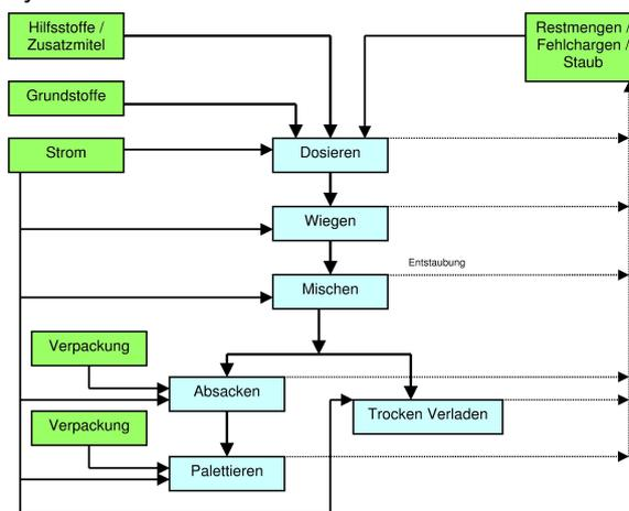
**Graphic 1:** Manufacturing process (green: input; blue: unit process)
