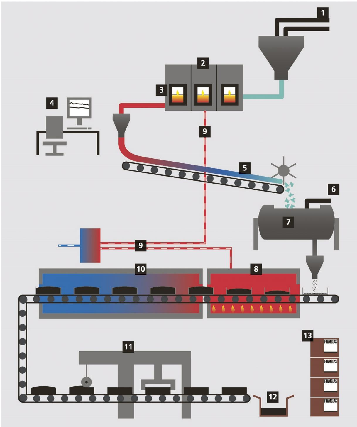
1 Mixing and batching of the raw materials: Recycled glass, feldspar, sodium carbonate, iron oxide, manganese oxide, sodium sulphate, sodium nitrate.
